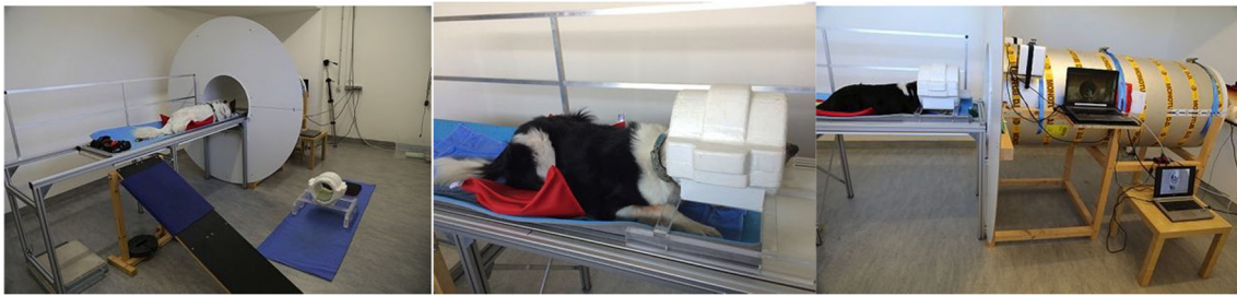
Fig. 3 Mock scanner: (Left) Dog lying on the movable table in front of the mock scanner. (Middle) Dog in prone position with head in the mock coil. (Right) Patient table, mock bore, loudspeaker, laptops, and display monitor in front of the bore
